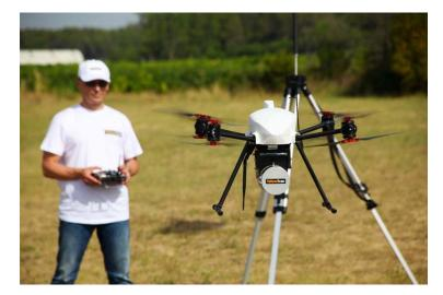
YellowScan Surveyor LiDAR Source:YellowScan.com
