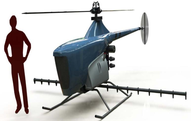
The configuration of the vehicle is focused at agricultural spraying with removable chemical tanks on either side of the fuselage. Although agricultural spraying is the primary application for this vehicle, it can easily be reconfigured to target other applications that require smaller payloads with longer flight times in the military, public safety, and remote sensing applications.
